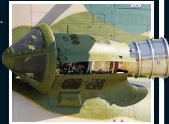
Above: A T55 turboshaft engine on a Japanese Air Self-Defense Force CH-47
